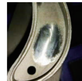
Gas turbine blade tip filling
