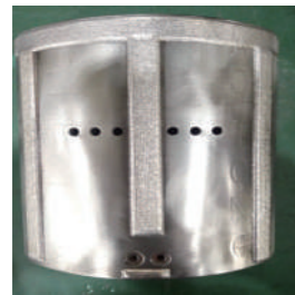
Pressure compensator wear repair
