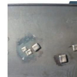
Seal tile repair
