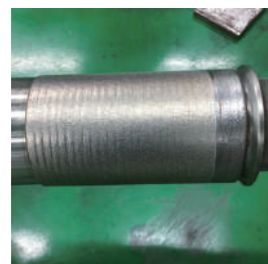
Laser repair of vehicle axle parts
