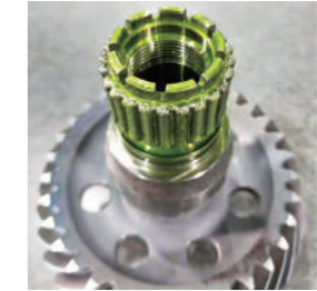
Repair of external spline shaft parts
