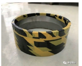
Salt spray test 1000h
