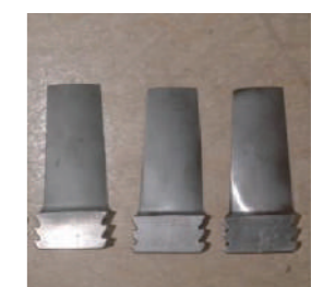
Steam turbine blade repair
